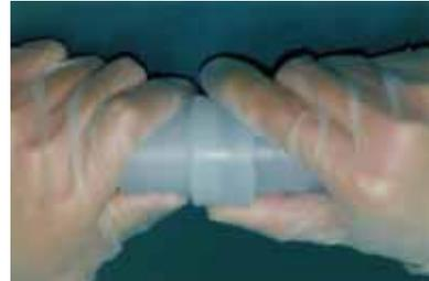
Make sure that the socket has been securely connected to the plug. (See Fig. 4 and photo.)
